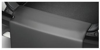
The rear bumper protection apron is fixed to the trunk deck with velcro. It protects the rear bumper when unfolded.
